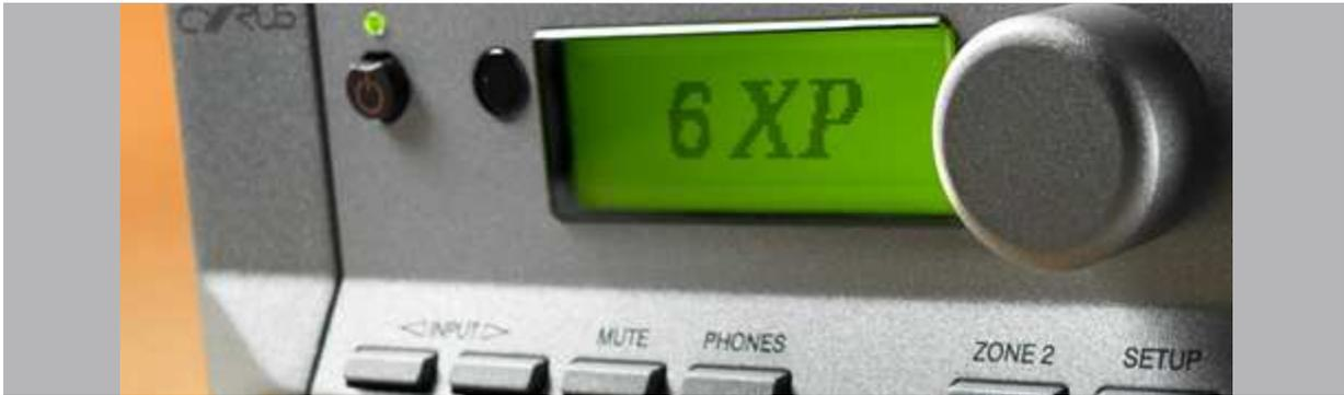
The Cyrus 6 XP is based on the Cyrus 8 XP but without the digital input option or a power supply upgrade port.
