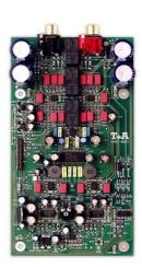
The D/A converter section is also of very sophisticated construction. Two of the best converters available are wired in double-mono mode for each channel. This design concept produces outstanding harmonic distortion, signal: noise ratios and dynamics. A special clock recovery circuit ensures perfect jitter characteristics.
