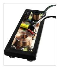
A completely new linear crossover layout, with the copper circuit paths arranged in the direction of electron flow, takes into account the potential for sympathetic and parasitic interactions among crossover components that may inject unwanted noise and distortions while allowing for more direct and efficient transfer of signal to the drivers which leads to a greater level of detail and purity.
