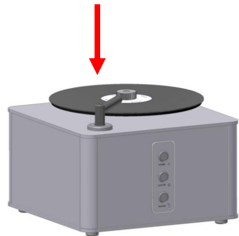
Pic. 4: Vacuum arm installation
