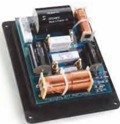
A hand built crossover from the 2-way models.
