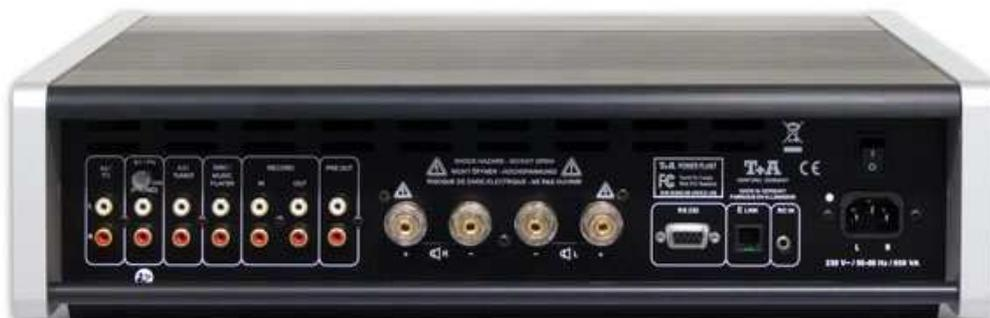
The amplifier features five high-quality inputs which are selected using gold-contact relays, and one of them can be fitted with the internal R-series PHE MM or PHE MC module to provide a phono input (earth terminal fitted as standard). REC OUT and PRE OUT are also present. The solid metal loudspeaker terminals are gold-plated and devoid of ferro-
