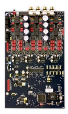
In the **SACD 1250 R** four of these converters are used for each channel in the form of our T+A quadruple converters, a further enhancement of the differential converter, which has been considered the last word in circuit design until now. The ground-breaking quadruple converter allows the machine to achieve values for total harmonic distortion, signal: noise ratio and dynamics which are genuinely extraordinary. The outstanding test results from all
