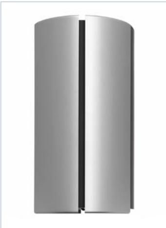
To maximise the inner volume of SUBSON, we profited from the stiffness of aluminum to realize a slim walled cabinet lacking in parallel walls, thereby avoiding deleterious internal standing waves. With a depth of only eight inches it is easy to understand why SUBSON is called the first „Flatwoofer,“ optimized for near-wall application.
